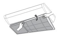
4. Clean the Air filter with a vacuum cleaner or soft brush. If dust is too heavy, then rinse it with running water and dry it in a ventilated area.
