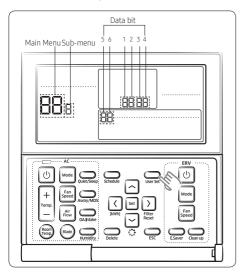
Press the User Set button. (Main Menu) will be displayed, and you can press the [^]/[√] buttons to select No. 8, which will set the Easy Tuning.
