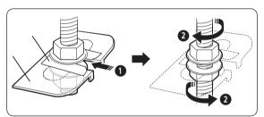
When installing the indoor unit, make sure it is not tilted toward front or back side.
